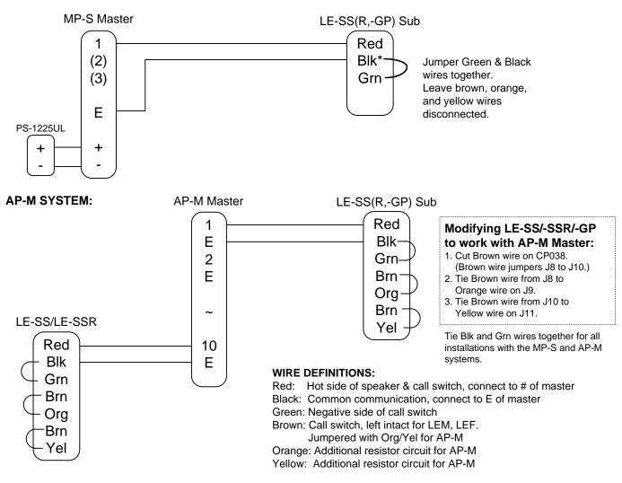
Intercom wiring must be run at least 20" away from any AC wiring, fluorescent lighting, dimmer switches, or any other electronic device that may cause interference.
